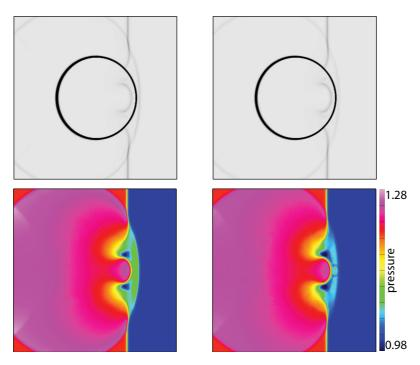
Figure 10: Simulation results for the shock-bubble interaction problem at  $t\!=\!0.31$ . The upper images show a numerical schlieren and the lower images the pressure. The results for the quasi-conservative scheme are on the left and the fully conservative scheme on the right.
