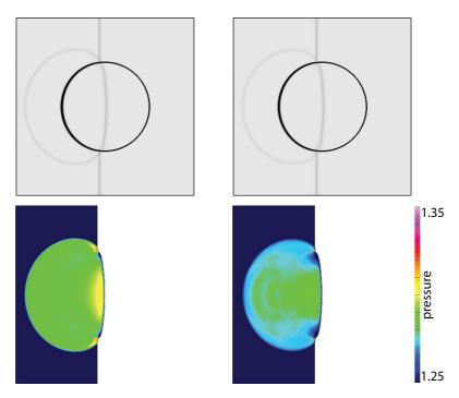
Figure 8: Simulation results for the shock-bubble interaction problem at  $t\!=\!0.2$ . The upper images show a numerical schlieren and the lower images the pressure. The results for the quasi-conservative scheme are on the left and the fully conservative scheme on the right.
