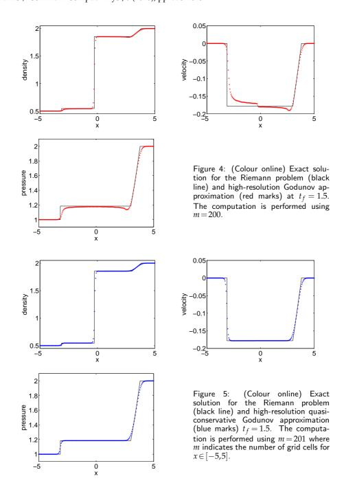
solution to the same problem using the quasi-conservative scheme (4.6). Clearly the solution behavior across the contact in the \*-regions is substantially better than the corresponding fully conservative results in Fig. 4. Also note that the shock lags behind the exact location for the fully conservative result, while the quasi-conservative result shows
