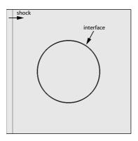
Figure 7: Initial conditions, shown as a numerical schlieren image, for the interaction of a shock with a bubble of higher density material.
