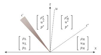
Figure 1: Typical structure of the Riemann problem in x-t space. Here the left and right acoustic waves are labeled with  $c^-$  and  $c^+$  respectively and the contact path with u. In this configuration, the solution consists of a left rarefaction and a right shock. The \*-state lies between the acoustic waves with the pressure and velocity remaining constant across the contact.
