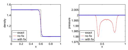
Figure 2: Numerical results for a contact only problem with the traditional Godunov scheme (4.2) as well as the scheme with energy corrected source term. Notice the deviation in pressure from UPV flow for the standard conservative scheme.
