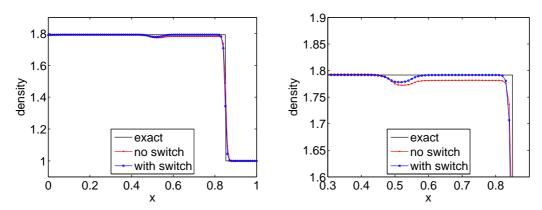
Figure 3: Approximations with and without the switch of Eq. (4.8). Both the full domain on the left and more detailed zoom on the right are show. Failing to turn off the source term near the shock results in a genuinely non-conservative approximation and convergence to a non-weak solution as shown in the figure.
