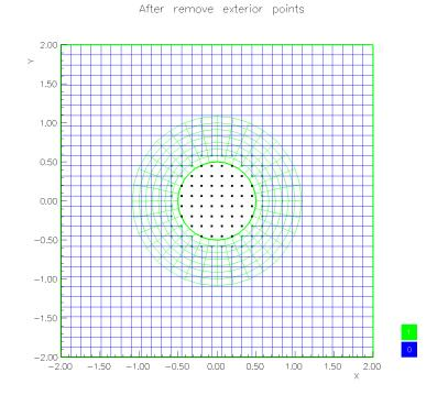
Grid after removing all exterior points. The exterior points are easily swept out after the hole boundary has been marked.
