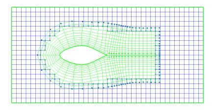
Figure 35: An overlapping grid using a c-grid makes use of the 'mixed boundary' option. A mixed-boundary is a boundary that is sometimes a physical boundary of the domain and sometimes an interpolation boundary.
