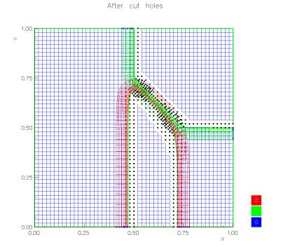
Grid after cutting holes. Physical boundaries are used to cut holes in nearby grids. The hole cutting algorithm will generate a barrier of hole points and interpolation points that bounds the entire hole region.
