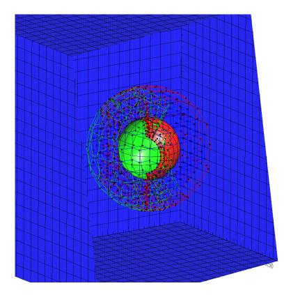
Figure 10: An overlapping grid for a sphere in a box. The interpolation points are also shown.
