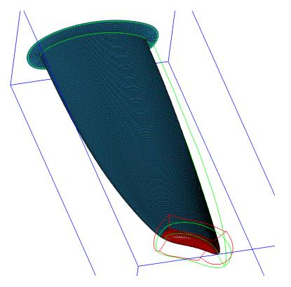
Figure 19: An overlapping grid for a wing with a Joukoswky airfoil and a *flat* tip constructed with the LoftedSurface Mapping.
