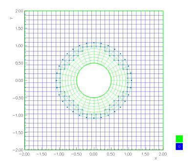
Finished grid after removing excess interpolation points.
