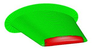
Figure 16: An overlapping grid for a three-dimensional wing with Joukowsky cross-sections and a rounded tip.
