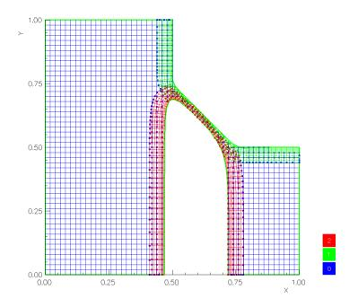
Grid after marking all (proper) interpolation.
