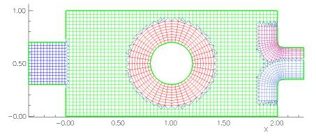
Figure 8: A hybrid grid for an inlet-outlet geometry.
