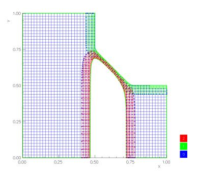
Finished grid after removing excess interpolation points.
