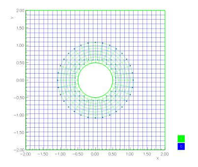
Grid after marking (improper) interpolation. These improper interpolation points need only lie inside another grid.
