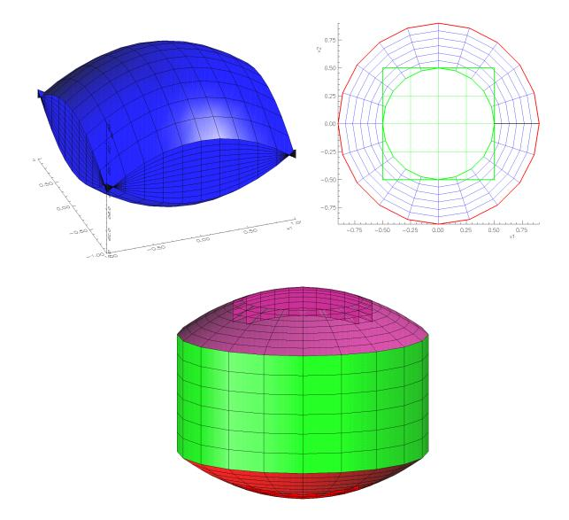
Figure 29: The DepthMapping (see bottom figure) is used to give a vertical dimension to mappings defined in the plane, depth.cmd. In this case a separate TFI mapping, top left, defines the vertical height function Both an annulus and a square (top right) are given a depth.
