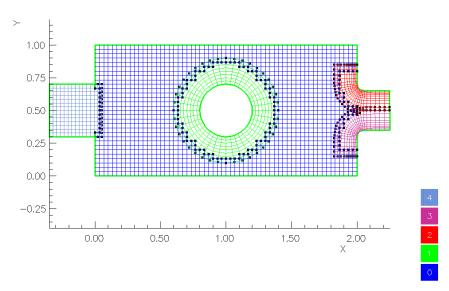
Figure 5: Inlet-outlet overlapping grid. To create this grid we had to prevent the background grid from cutting holes in the two inlet grids (on the right) and the outlet grid on the left. The outlet grid was also prevented from cutting holes in the background grid.
