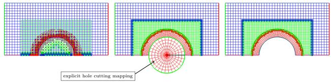
Figure 38: Explicit hole cutting is used for a half-annulus in a rectangle with a refinement grid. Left: default hole cutting algorithm fails since the background grid and refinement grid can interpolate from one another inside the half-annulus cavity. Middle: An annulus mapping is used to explicitly cut holes in the cavity. Right: final grid.
