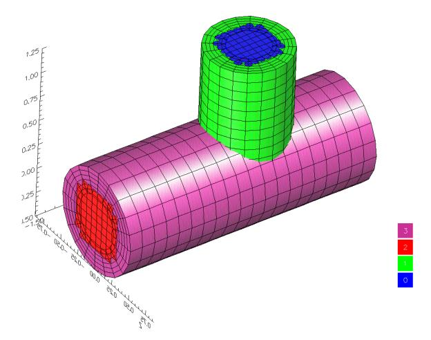
Figure 12: An overlapping grid for two intersecting pipes
