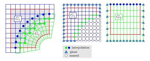
Figure 2: Left: an overlapping grid consisting of two structured curvilinear component grids,  $\mathbf{x} = G_1(\mathbf{r})$  and  $\mathbf{x} = G_2(\mathbf{r})$ . Middle and right: component grids for the square and annular grids in the unit square parameter space  $\mathbf{r}$ . Grid points are classified as discretization points, interpolation points or unused points. Ghost points are used to apply boundary conditions.
