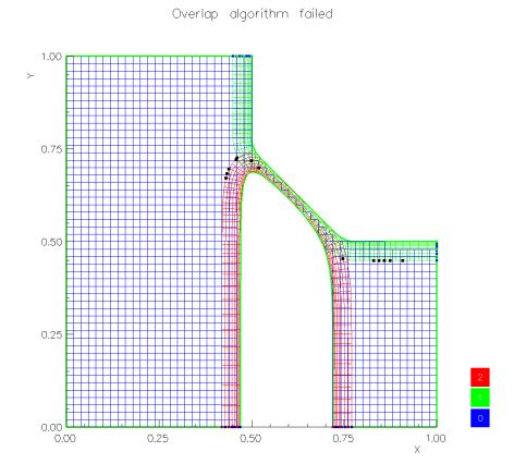
Figure 40: An example showing the failure of the overlapping grid algorithm when there is insufficient overlap. We have tried to use explicit interpolation for the two-dimensional valve. The algorithm fails and plots the offending points with black marks.
