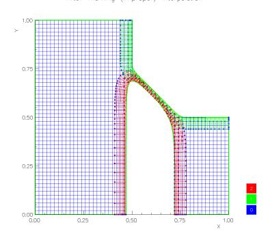
After marking (improper) interpolation
