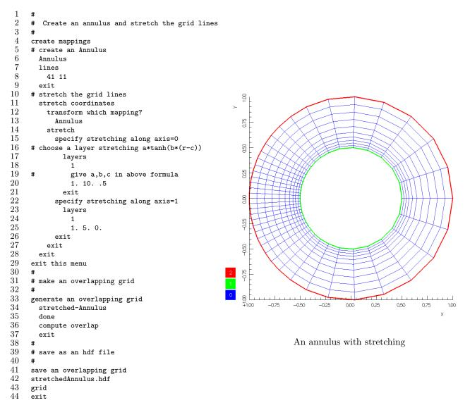
For the pundits: The stretched annulus is a StretchTransform Mapping which is a composition of the StretchedSquare Mapping and the Annulus Mapping. The StretchedSquare uses the Stretch Mapping where the actual one dimensional stretching functions are defined.
