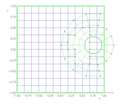
Figure 46: When two boundaries are nearby to one another the overlapping grid algorithm ensures that enough interior grid-points remain next to the boundary points to allow the boundary point to be discretised. While not very accurate this approach at least allows a grid to be built.
