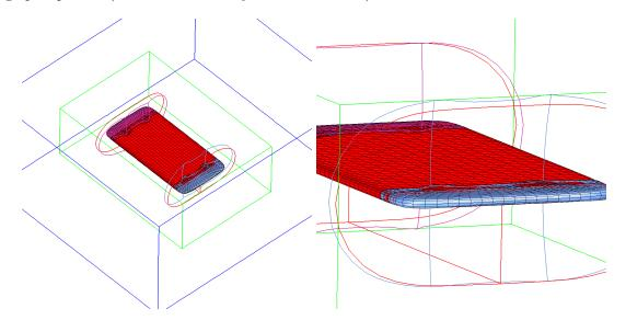
Figure 17: An overlapping grid for a three-dimensional flat-plate wing in a box.
