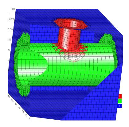
Figure 25: A JoinMapping is used to join two cylinders, joinTwoCyl.cmd. To create the deformed cylinder the JoinMapping first computes the curves of intersection between two intersecting cylinders. Four TFIMappings are then generated to represent each face of the deformed cylinder and finally another TFIMapping is used to blend these four surface TFIMa
