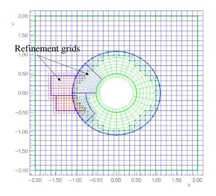
Figure 47: When refinement grids are added to an overlapping grid, the updateRefinement function should be called in order to compute a valid grid.
