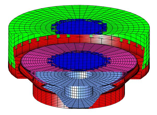
Figure 14: An overlapping grid for a three-dimensional valve.
