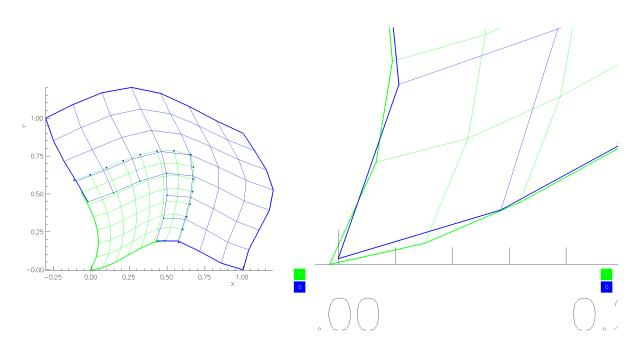
Figure 43: An overlapping grid testing the mismatch problem, created with mismatch.cmd. The refinement grid is artifically translated so that the two boundaries it shares with the base grid do not match. The figure on the right is a magnification of the lower left corner, before the overlap algorithm was applied.
