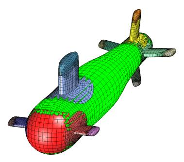
Figure 26: An overlapping grid for a submarine created with sub.cmd. The submarine hull is defined as a body of revolution from a spline curve. The sail and fins are created initially with the CrossSectionMapping. The JoinMapping is used to join these appendages to the submarine body.
