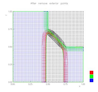
Grid after removing all exterior points. The exterior points are easily swept out after the hole boundary has been marked.
