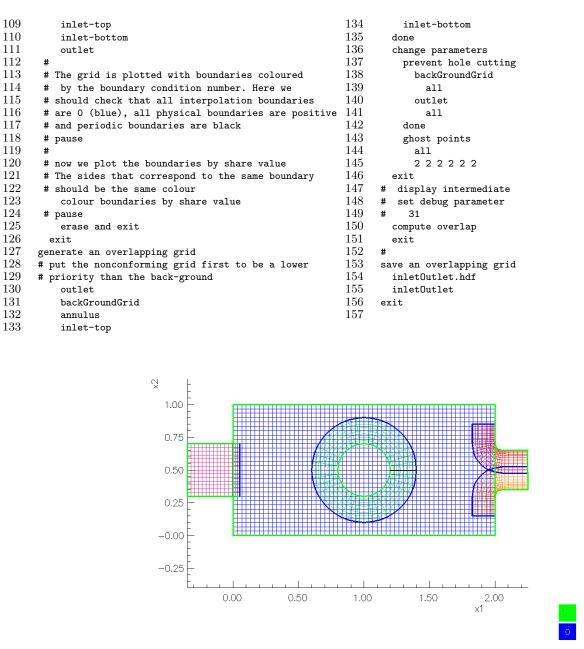
Figure 3: Inlet-outlet mappings plotted from the "view mappings" menu, showing boundary condition values. Physical boundaries have a positive value (1=green), interpolation boundaries have a value of zero (0=blue) and periodic boundaries have a negative value (shown in black).
