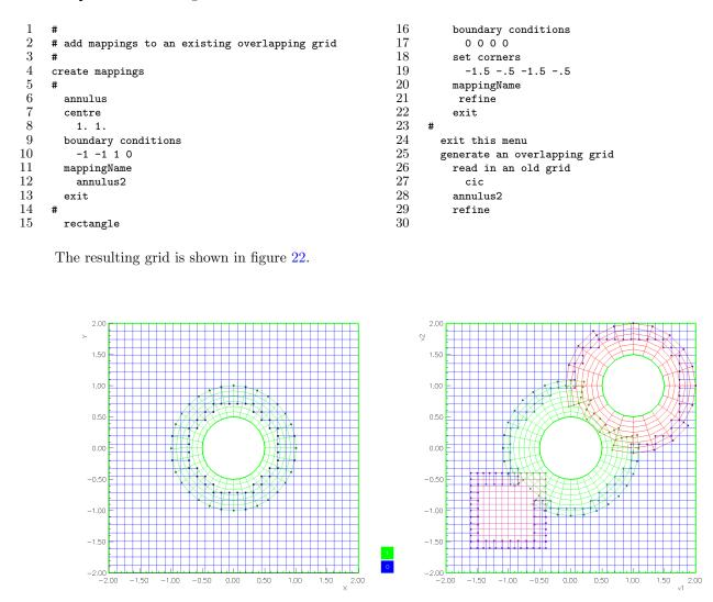
Figure 22: Ogen can be used to incrementally add new grids to an existing overlapping grid. Left: The initial overlapping grid. Right: overlapping grid after adding two new component grids
