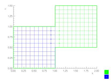
Figure 37: An overlapping grid for two blocks makes use of the 'mixed boundary' option.
