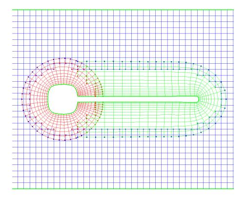
Figure 28: A mast is attached to a sail. The inner boundary curves are defined from splines under tension while the component grids are generated with hyperbolic grid generation mastSail2d.cmd
