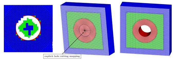
Figure 39: Explicit hole cutting is used for a cylinder in a box with a refinement grid. Left: default hole cutting algorithm fails since the background grid and refinement grid can interpolate from one another inside the cylinder cavity. Middle: A cylinder mapping is used to explicitly cut holes in the central cavity. Right: final grid.
