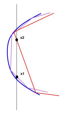
Figure 42: The points of intersection of a ray with a surface covered by two overlapping grids. If the ray is nearly tangent to the surface then the two points of intersection may not be very close together.
