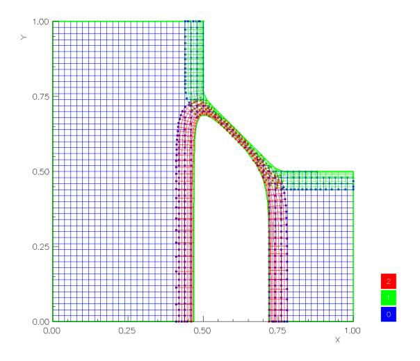
Figure 6: An overlapping grid for a valve
