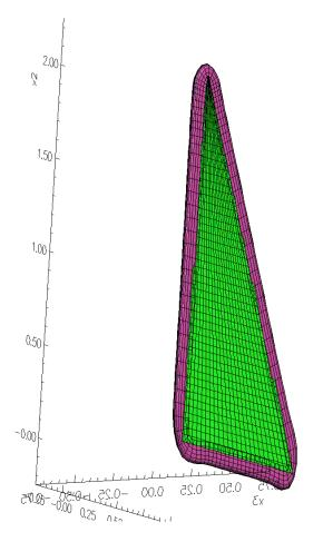
Figure 31: Grid for a 3d triangular sail. The SweepMapping is used to generate a grid around the edge of the sail, triSail.cmd
