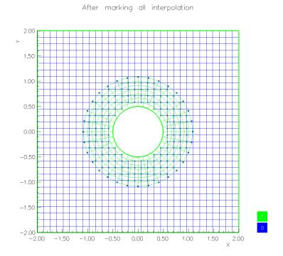
Grid after marking all (proper) interpolation. We have attempted to interpolate discretization points on each grid from grids of higher priority.
