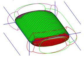
Figure 15: An overlapping grid for a three-dimensional wing in a box.
