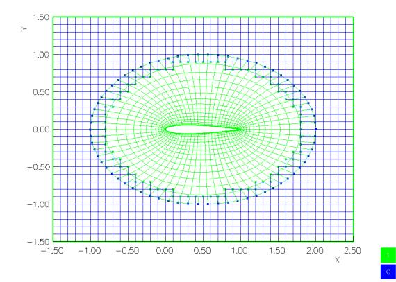
Figure 7: An overlapping grid for a NACA0012 airfoil
