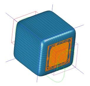
Figure 18: An overlapping grid for the region exterior to a box constructed with the LoftedSurface Mapping.
