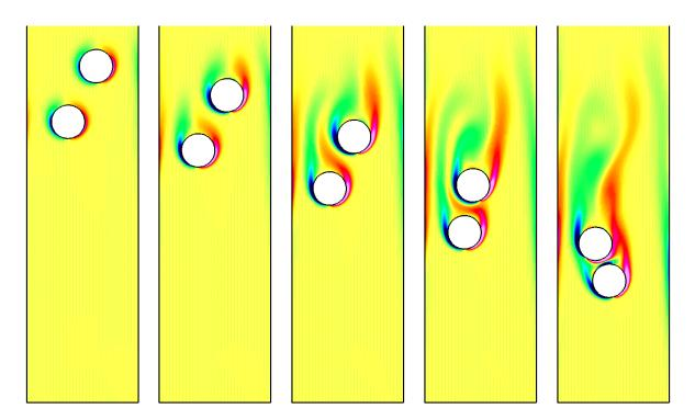
Figure 11: Two drops falling in an incompressible flow, contour plots of the vorticity. The upper drop wants to "draft" in behind the lower drop where the pressure is lower.
