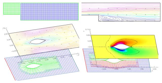
Figure 8: Incompressible flow past a backward facing step, a C-grid and an H-grid.
