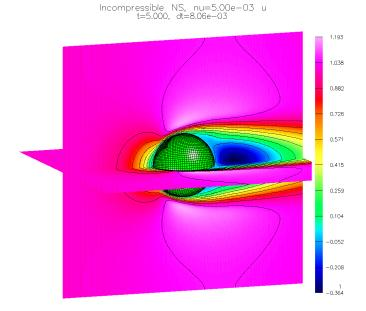
Figure 9: Incompressible flow past a sphere.
