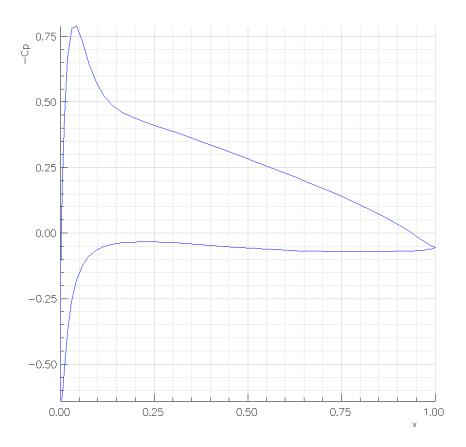
Figure 13: The area.C program can be used to read a show file generated by cgins and compute the coefficient of pressure on the surface of a body.
