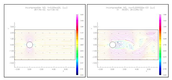
Figure 2: Incompressible flow around a cylinder. Left: the initial conditions are obtained by projecting a uniform flow, (u, v) = (1, 0). Right: the solution at time t = 40.
