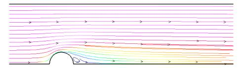
Figure 7: Incompressible axisymmetric flow past a sphere.
