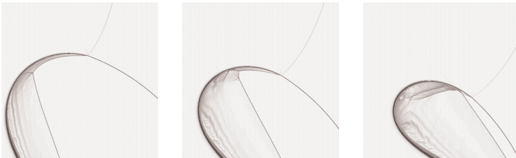
Fig. 19 Spherical cavity, M_s = 2.0 . Numerical schlieren images in the cavity at times t = 0.052 (left), t = 0.060 (middle) and t = 0.067 (right).
