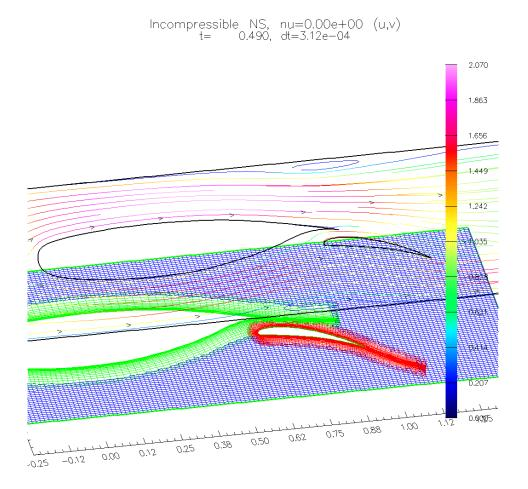
Figure 2: plotStuff can be used to plot more than one quantity on the same figure; here streamlines and a grid are plotted. This plot used an option in the grid-plotter to change the height of the grid. This computation was performed by the **OverBlown** solver.
